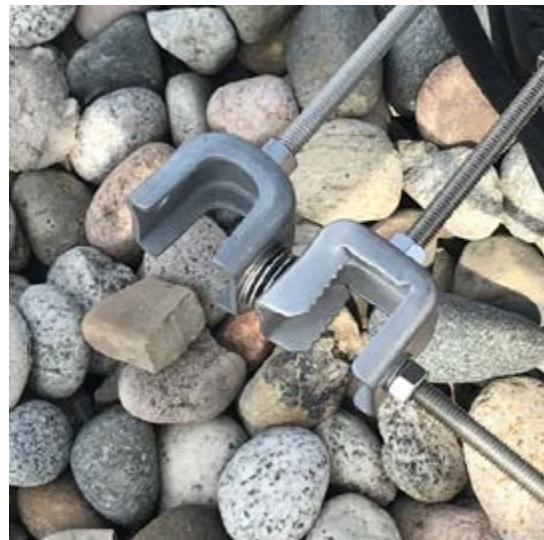
STACK OF LOOSE WASHERS INSTALLED ON SUPPORT
