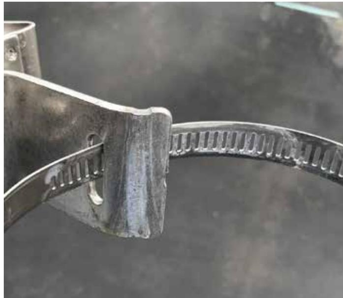
**Figure 9:** Galvanic corrosion found on stainless-steel site hardware
