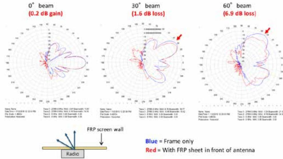
While the antenna pattern is good at 0° and has some degradation at 30°, the 60° pattern is clearly degraded. The next set of antenna patterns is with a flat sheet of FRP located 3.45" from the face of the array. The plots show significant amounts of reflection that severely distort the antenna patterns at all beam angles.
