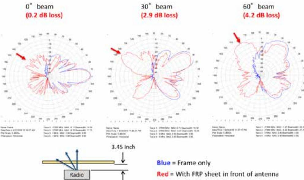
Now the antenna patterns are taken with the flat sheet of FRP at 30° and 60° angles to the face of the array. Again, there is significant distortion of the antenna patterns.
