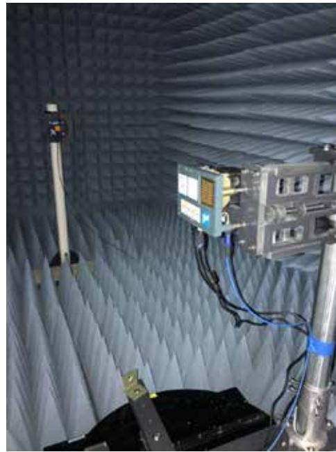
First the antenna patterns were taken with a flat sheet of FRP directly against the face of the array.
