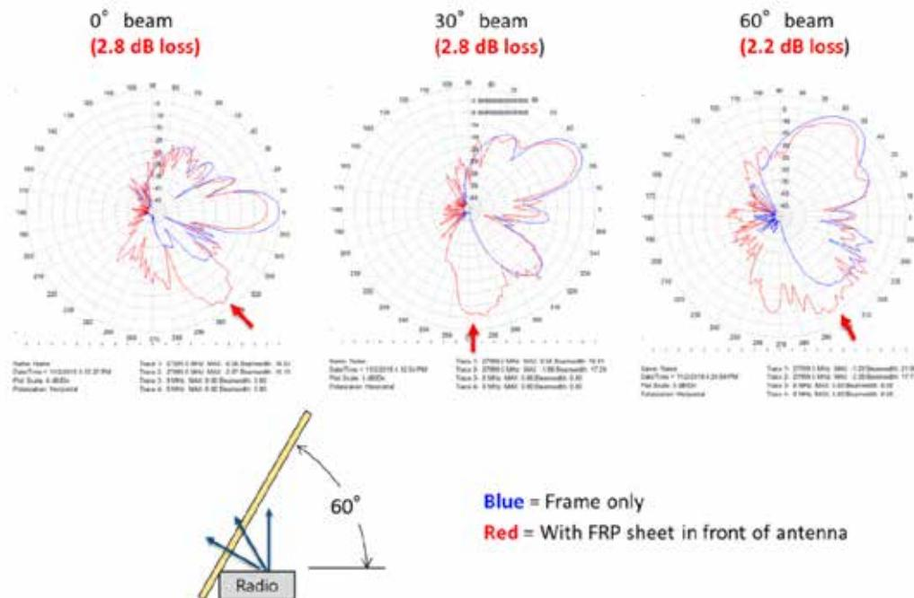
In some instances, an antenna might be shooting out through a corner of the rooftop concealment to maintain the desired azimuth. Below are antenna patterns with the antenna shooting through the FRP joined at a 90° angle. First with the corner unreinforced and then reinforced by a 4x4 angle. Again the antenna patterns show significant degradation.
