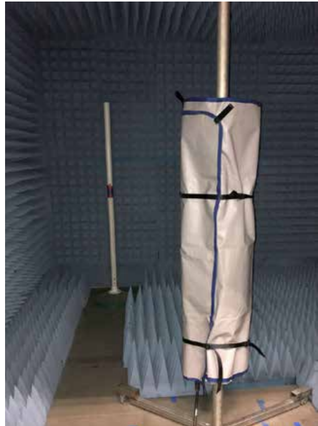
Antenna Wrapped in PIM Blanket
